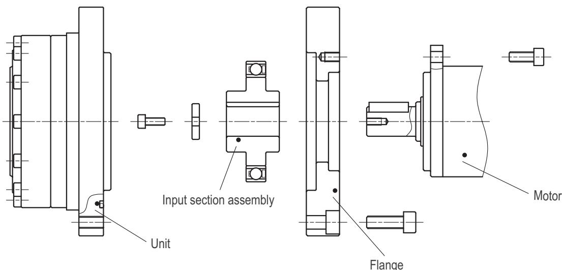
\* This model is not directly attached to a motor. Necessary fixtures are to be prepared at the customer side.
