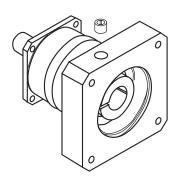
G. Re-install the access hole plug into the motor adapter plate. Assembly is complete.
