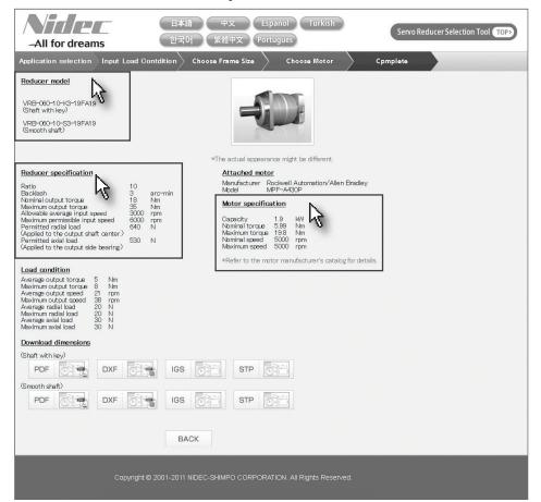
The resulting Load Condition can be helpful for sizing other related machine components
