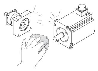
D. Clean and de-grease the motor mounting surface and shaft, as well as the gearbox mounting surface, input hub bore, and shaft bushing (if included). This cleaning is very important for the shaft and bushing, to prevent slip during motion.
