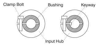
B. Carefully align the shaft bushing (if included) so that the opening in the bushing aligns with the opening in the input hub. It is also recommended that the motor shaft keyway (if present) aligns with the opening in the input hub clamp.
