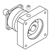
G. Re-install the access hole plug into the motor adapter plate. Assembly is complete.
