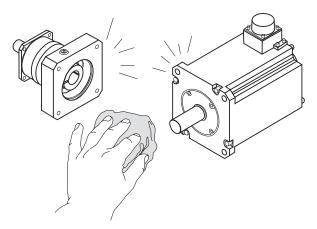
D. Clean and de-grease the motor mounting surface and shaft, as well as the gearbox mounting surface, input hub bore, and shaft bushing (if included). This cleaning is very important for the shaft and bushing, to prevent slip during motion.
