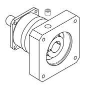
A. Remove the access hole plug, allowing access to the motor shaft clamp.
