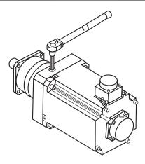
F. Tighten the gearbox input shaft clamp bolt to the proper torque using a torque wrench (see Table B).
